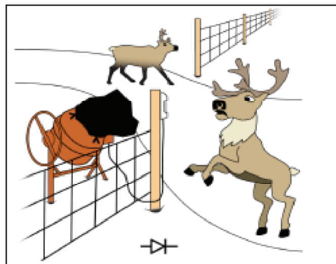
Fig. 2. When the reindeer enter the sector of the motion detector, the mixer starts running and frightens the reindeer back. As there is no motion detector to the opposite direction, the reindeer from the neighboring herding district can enter unhindered into their new owner's territory.
