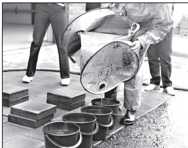
Fig. 4. To measure the final volume, the crushed barrel was filled with water. Result: 35 liter.
