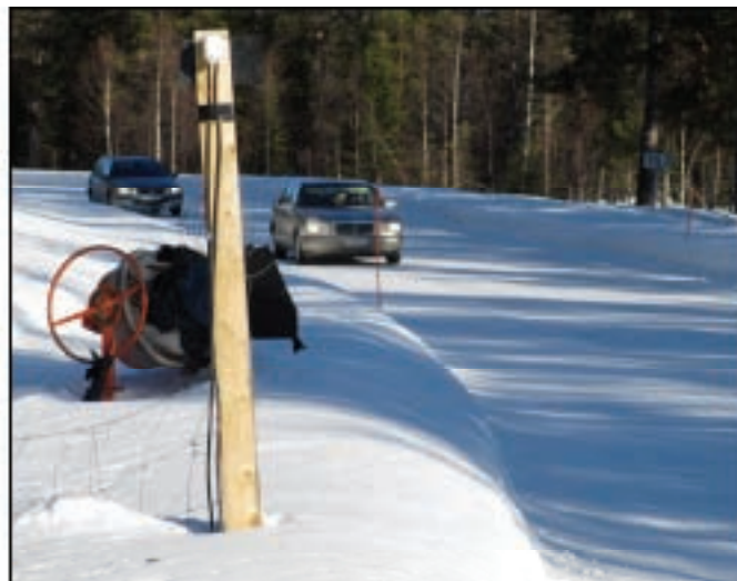
Fig. 1. A roadside reindeer diode consists of a motion detector (in the foreground) and an ordinary concrete mixer (behind).
