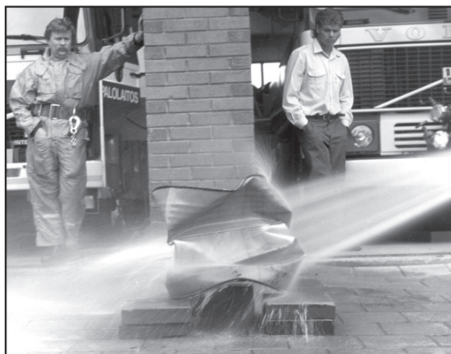
Fig. 3. A cold spray of water cools the barrel and condenses the steam inside. Air pressure crushes the barrel rapidly.
