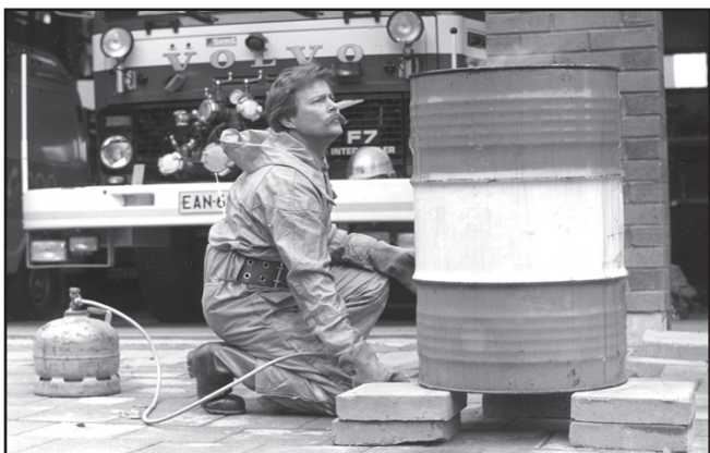
Fig. 2. Fireman Pertti Siren watches steam rise from the barrel while he heats the bottom with a torch. After 4–5 min of boiling, the cap was screwed on tightly.
